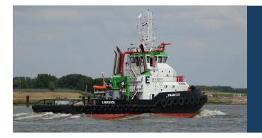
Name Port of Registry Flag Vessel Type Year of Build Class Bollard Pull Owner E-NINE Limassol Cyprus Shoalbuster 3612 2010 Bureau Veritas 70 tbp Operator : Emar Offshore Services B.V.
